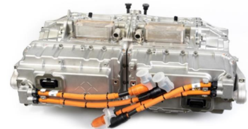
DUAL MOTOR DRIVE UNIT (REAR)
