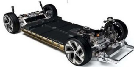
Lucid "Skateboard" EV Platform In-house design, underpinning Lucid's "Space Concept"
