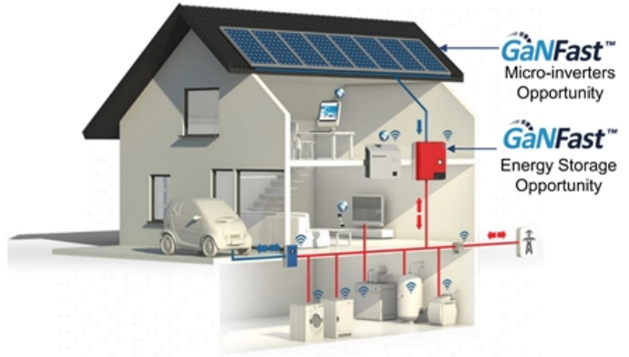
Power is converted from DC low-voltage solar panels to AC high-voltage to power your home or the power grid and to high-voltage DC stored in a battery (energy storage).
