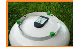
Connected Gas Tank Monitors
