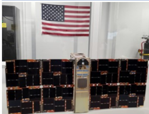
GEOstare SV2 nanosatellite outfitted with LLNL payload, launched May 15, 2021.
