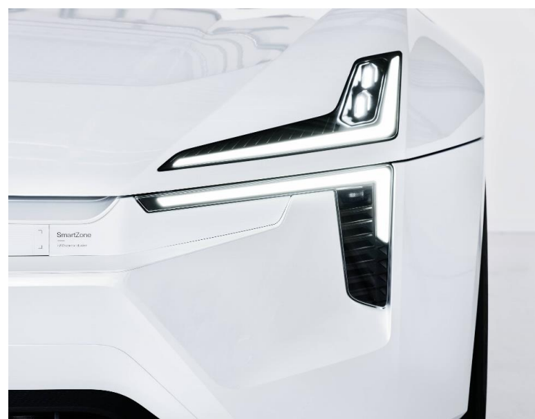
Signature Headlights and SmartZone with ADAS sensors
